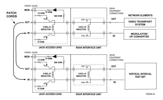
Figure 29. Insertion of Test Signal
